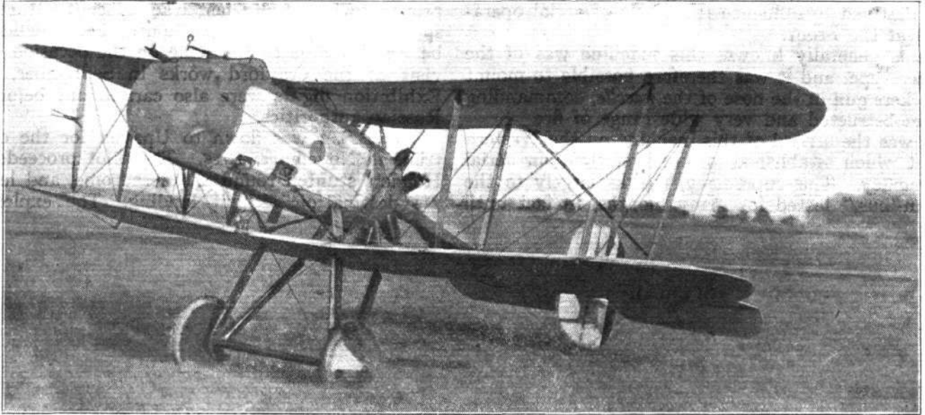
THE VICKERS F.B. 12 PUSHER SCOUT. —This particular machine is fitted with a 100 h.p. Gnome, but others of the same type were fitted with 80 h.p. and 110 h.p. Le Rhones and 100 h.p. Anzani
